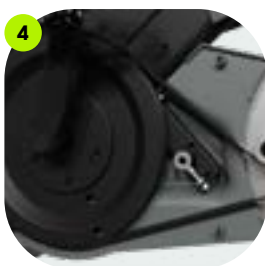
Double bearing belt tension system
